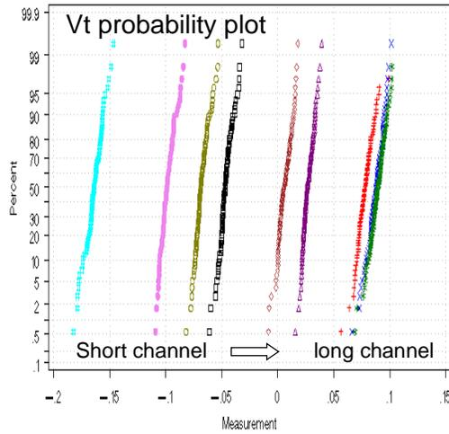
Long channel Vt range only 35 mV on a 300 mm wafer!
