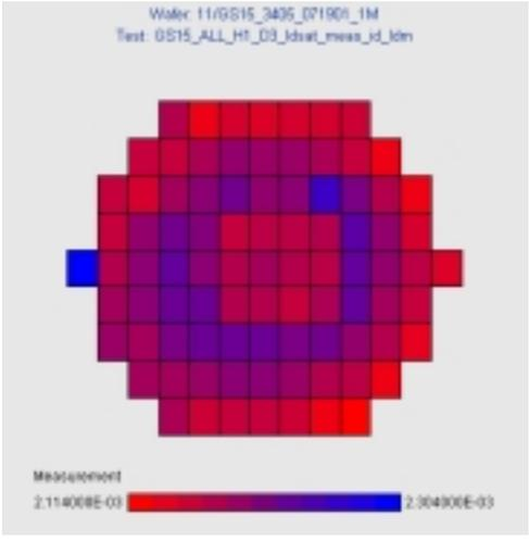
Idsat wafer map for checking pattern dependencies.
